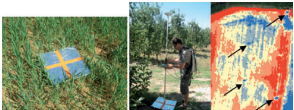
Fig. 10. Aluminium targets – Position measurement – Targets seen as cold points on thermal image.
