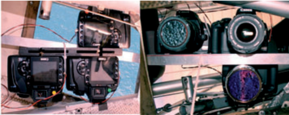
Fig. 7. Examples of visible and modified near infrared cameras on an ULA.
