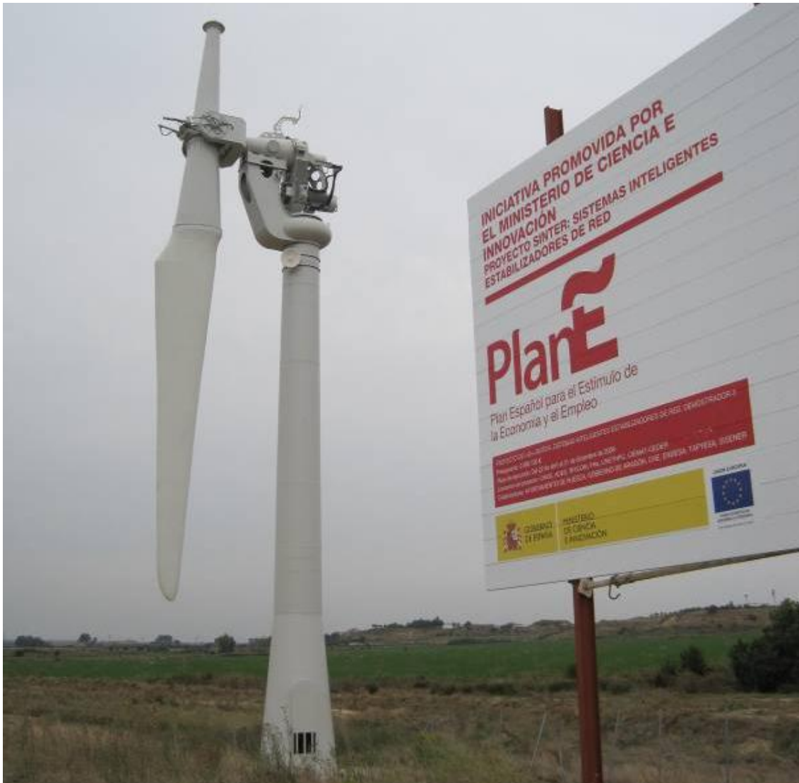
Ilustración 9. 250 kW single-bladed ADES wind turbine with oscillating rotor and powertrain pendulum.
